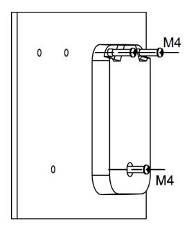
Use screws that are suitable for the mounting surface structure.
