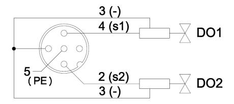
c) PNP Input and output signal – 1 connector connects 1 DI and 1 DO. LKHA-08UP-M12 support this connection.
