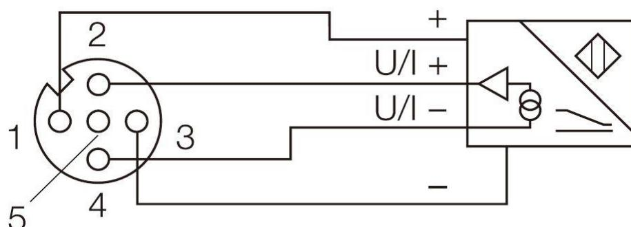
d) Current output- 1 connector connects 1 current output, FEEC-04UA-M12-T supports this connection.
