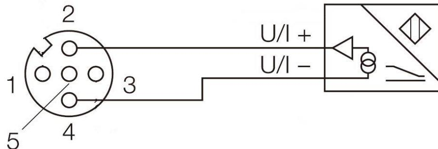
e) Voltage output- 1 connector connects 1 voltage output, FEEC-04UA-M12-T supports this connection.
