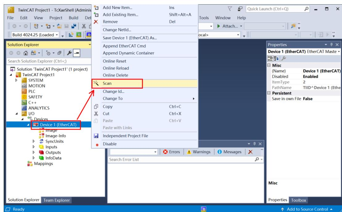
2) If the gateway is connected to PLC properly, the system can automatically search the Slim67 analog module and see the specific module connection.
