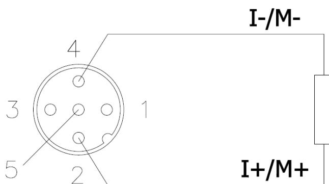
g) Thermocouple signal — 1 connector connects 1 thermocouple signal,
