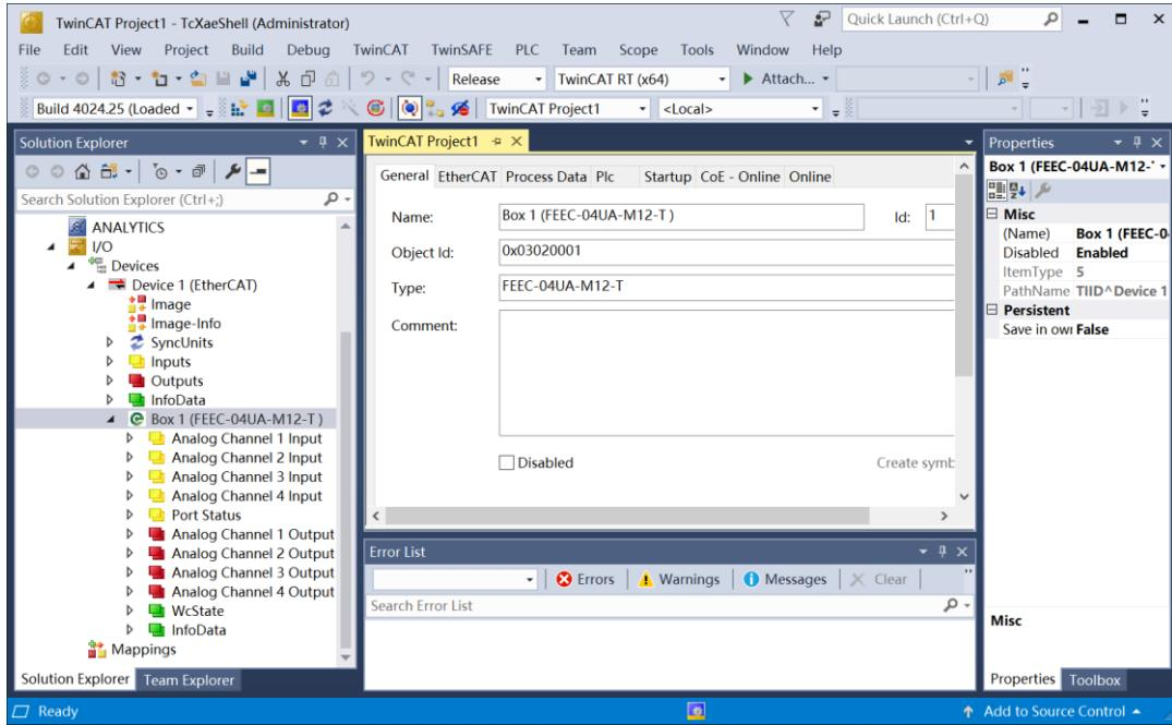
3) To configure the input/output type and specific range of the module, double-click to enter the “Startup” tab, and double-click the corresponding channel to open the attribute setting window.
