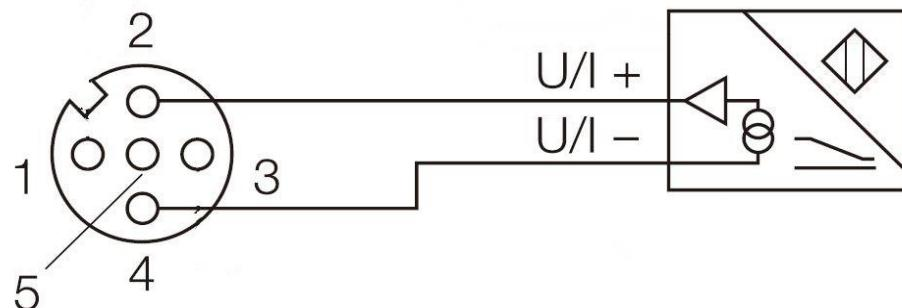
f) Two-wire thermal resistance signal — 1 connector connects 1 two-wire thermal resistance signal, FEEC-04UA-M12-T supports this connection.
